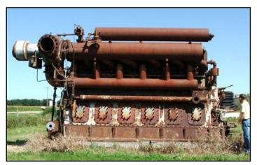
The picture above is of the third diesel/ natural gas engine purchased in 1945. This was a 1200 horsepower engine. This Worthington engine was 15'-7" long, 5'-3" wide and 11' tall. This mammoth was also six-cylinder. It produced 840 kilowatts at 1050 RPM. Note the relative size of the engine to the size of Gary standing off to the side.
