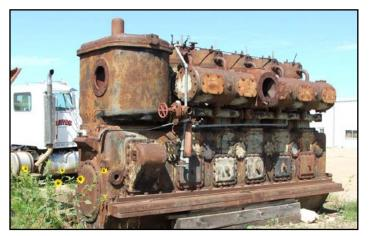
The picture above is of one of two 525 horsepower diesel engines. This Fairbanks Morse motor is 15'8" long, 5'4" wide and 9'tall. It is a five-cylinder giant that produced 357.6 kilowatts at 447 RPM. This is one of two engines that were placed in the original power plant, which was built in 1931. The other 525 horsepower engine was sold as scrap metal.
